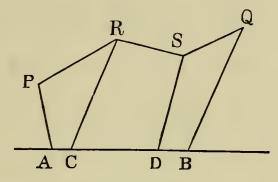
B or to the left of A, this will be no longer the case. We may agree to consider the projection of a line to be equal to its length multiplied by the cosine of the angle which it makes with the second line, those angles being always taken which are formed by the successive lines PR, RS, SQwith AB towards the same part. Thus if D come to the left of C, the angle between RS and AB will be obtuse, and the projection of RS will be negative. And since
